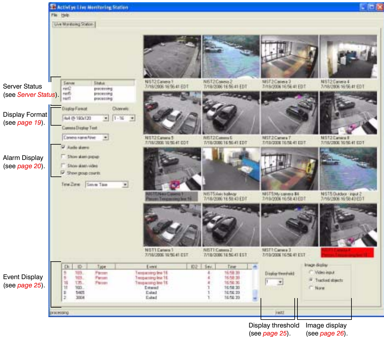
Figure 1-2 Live Monitoring Station, Showing Areas of Interest
