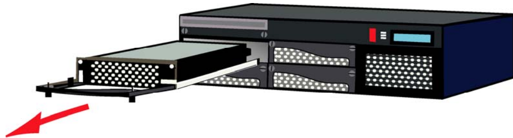
Fig. 5-3. Removing a Drive on a Rapid Eye DVR.
