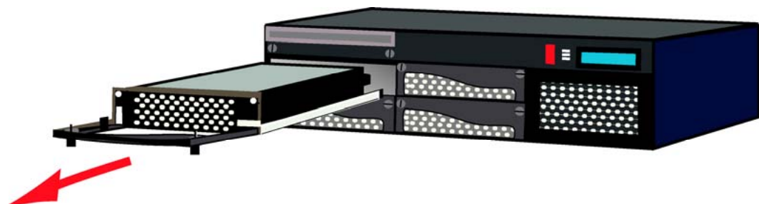
Fig. 41. Pull to remove a mounted hard disk from a unit; push to insert. Remove the front cover of the unit beforehand.
