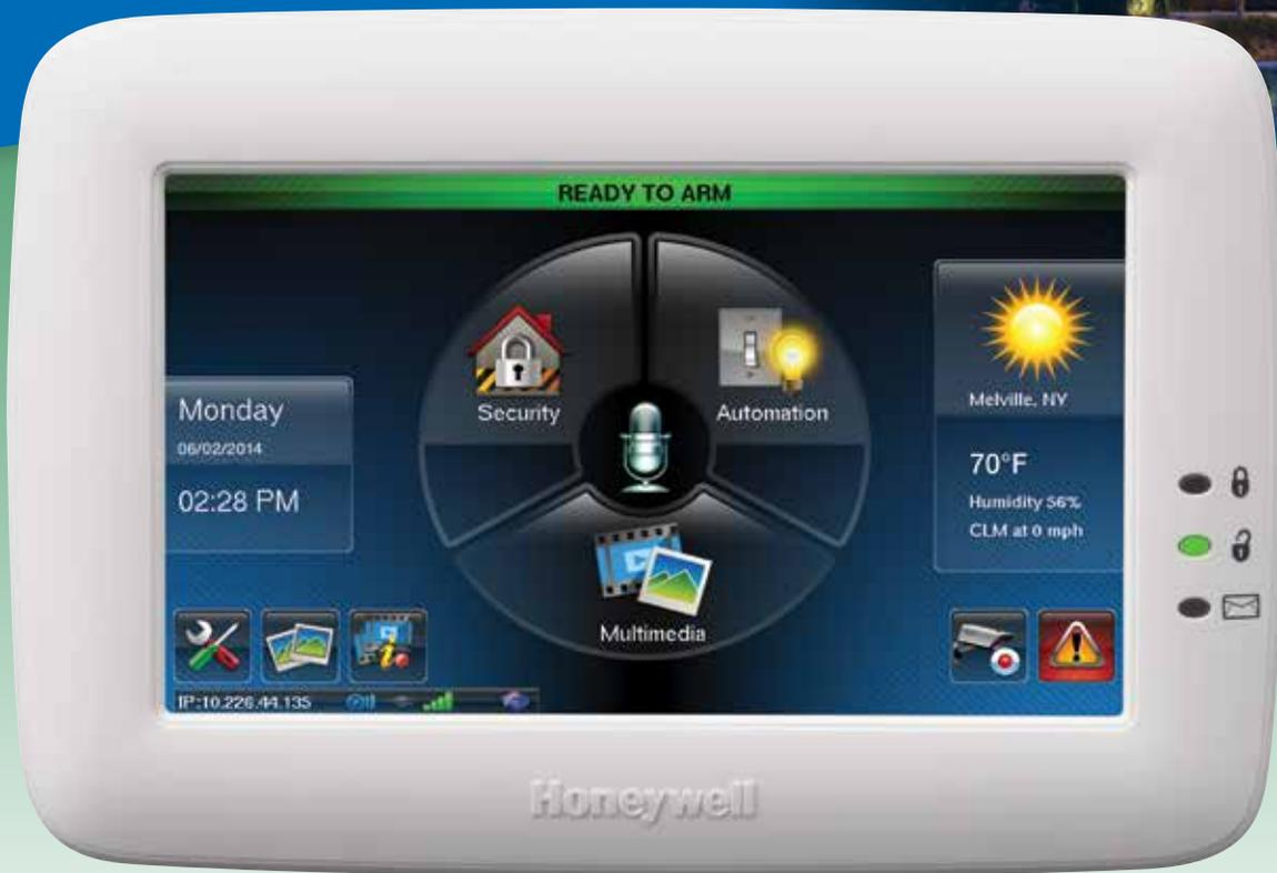
**Honeywell's Tuxedo Touch functions as an advanced home security and automation controller, video camera/recorder and voice-enabled system.**
